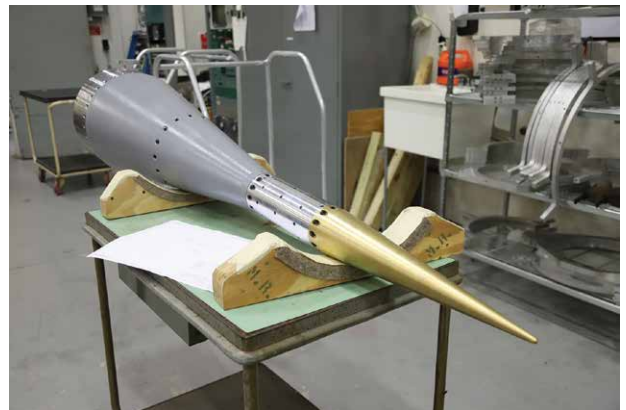
MesOrion 4-inch payload. NASA Photo/Berit Bland
